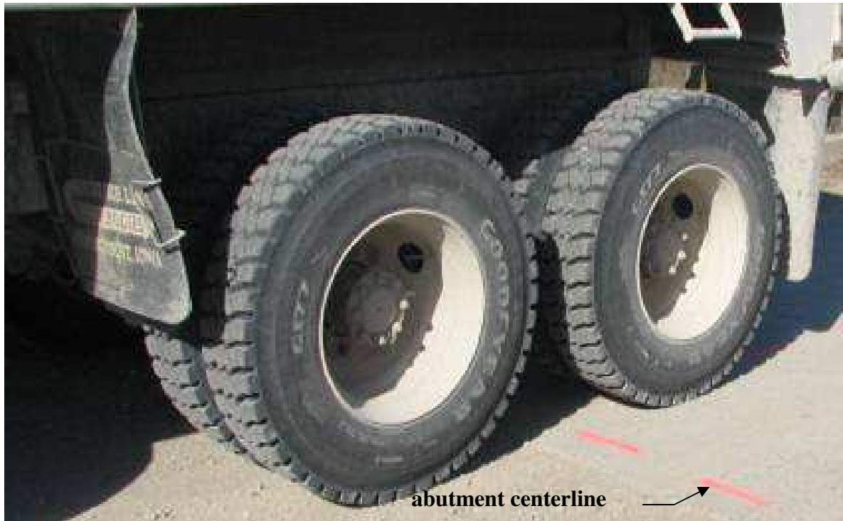
Figure 3.11. BCB Truck Tandem Centroid Centered Over Abutment.
